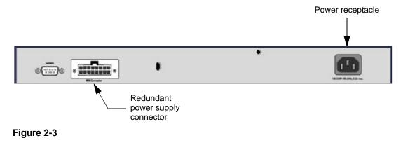
You can connect an external DC-to-DC power supply unit to the switch to provide redundant power in case the primary power supply fails. To connect a redundant power supply (RPS) unit to the switch, first turn off the switch. When the power is off, you can remove the cover plate and connect the RPS unit to the switch. After all connections are completed, apply power to the switch.
